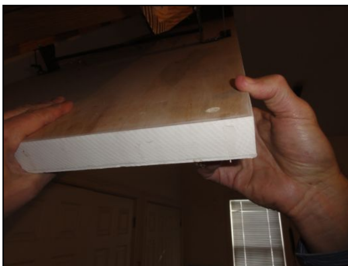
Fire barrier broke with pull down steps
